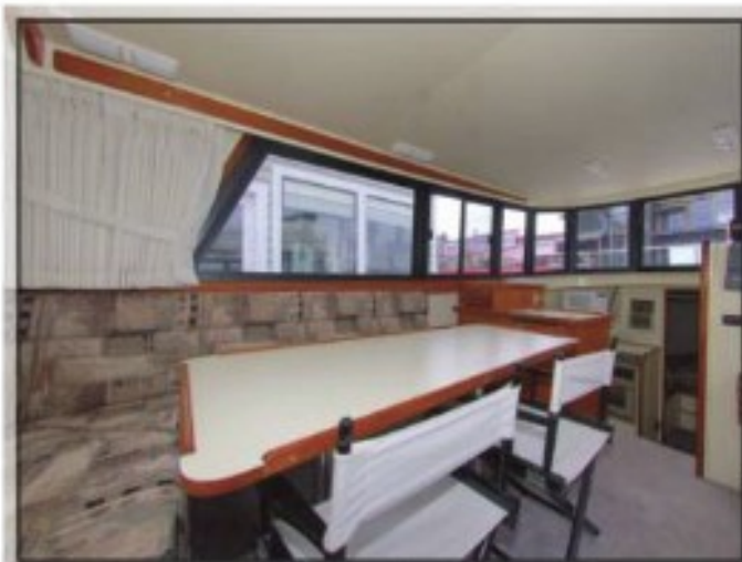
A dinette and hi-lo table in the salon converts into a second double berth.
