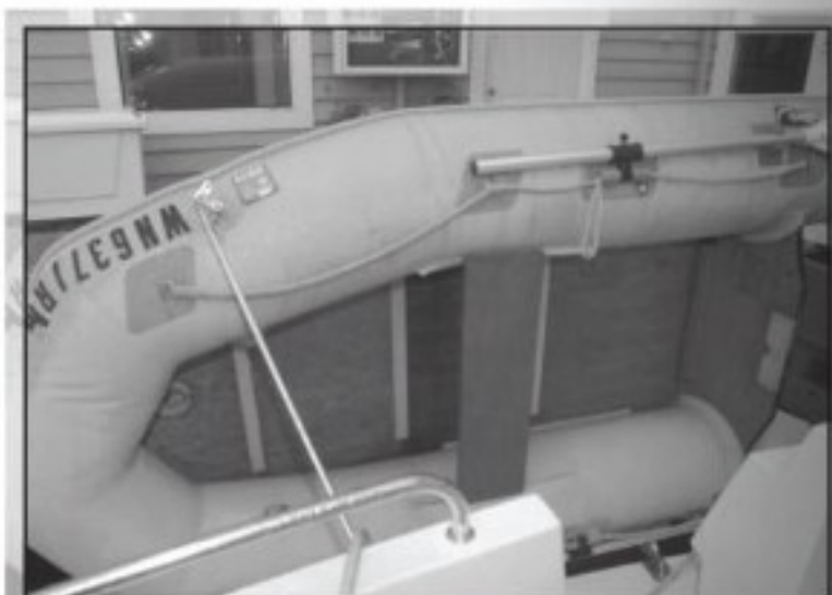
An Achilles inflatable on snap davits is easy to deploy.
